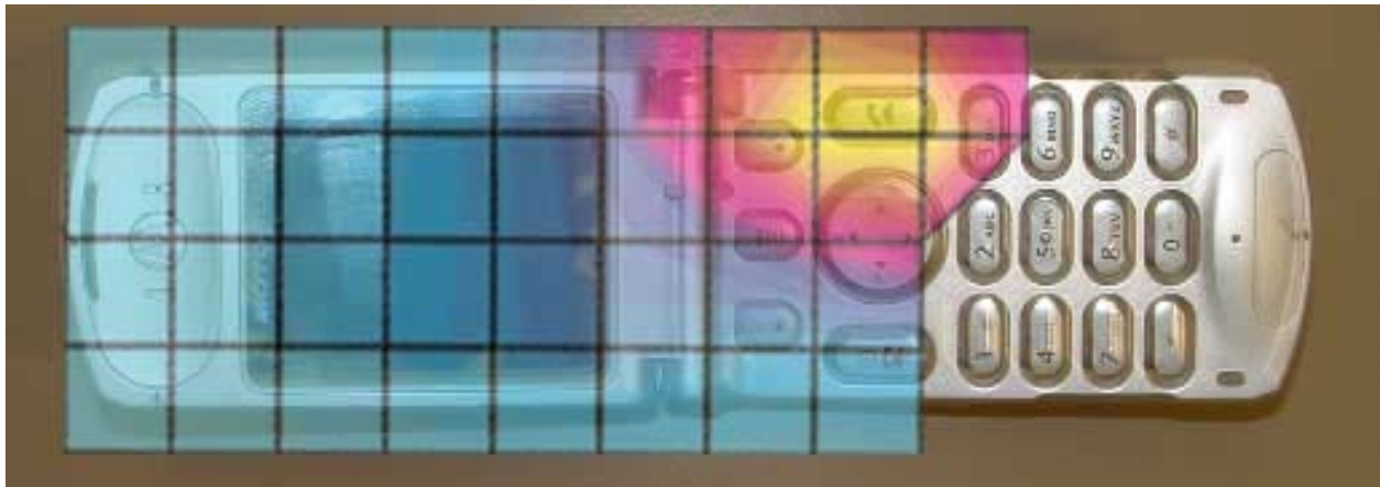
Figure 1. Typical 800MHz Left Head Adjacent Contour Overlaid on Phone with Antenna Fixed (Cheek Touch)
