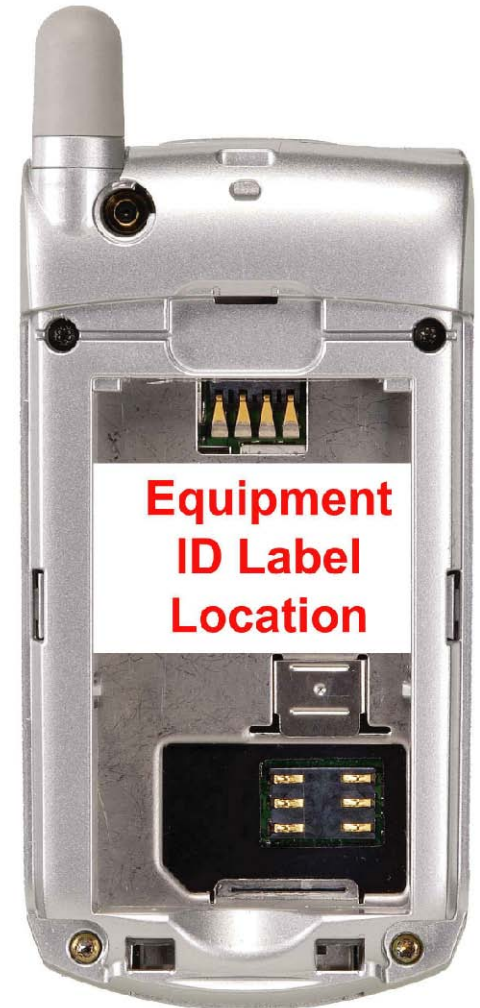
Rear View with Battery Removed to Show Equipment ID Label Location
