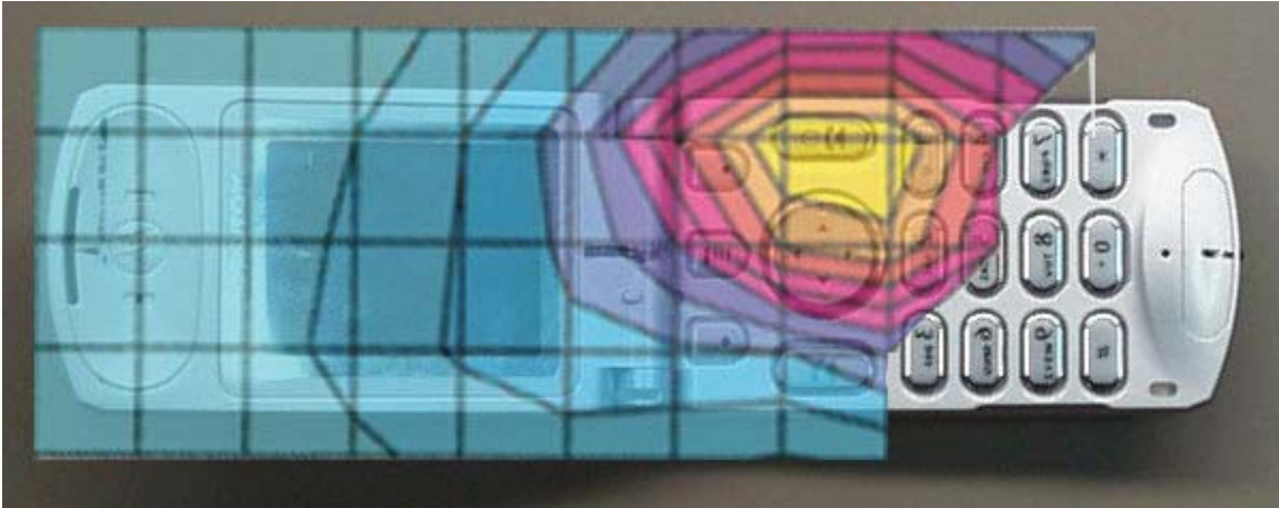
Figure 1. Typical 800MHz Head Adjacent Contour Overlaid on Phone (Cheek Touch)
