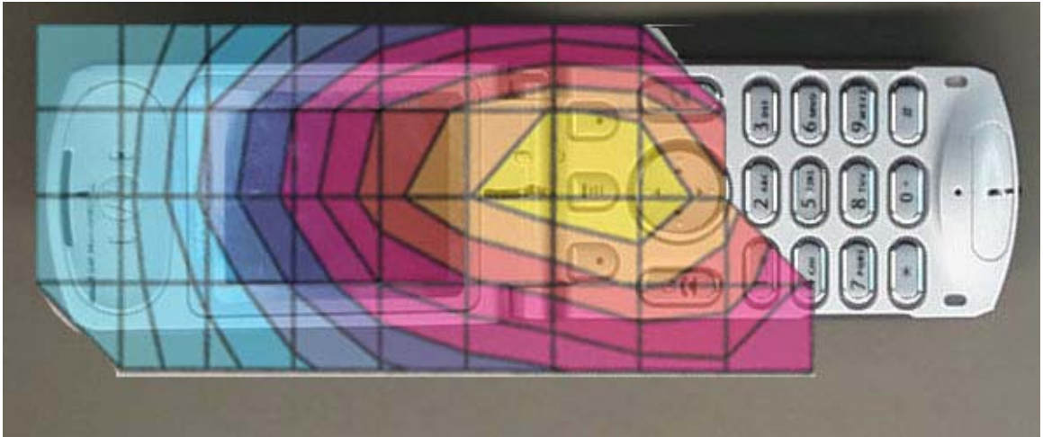
Figure 3. Typical 800MHz Head Adjacent Contour Overlaid on Phone (15 ° Tilt)
