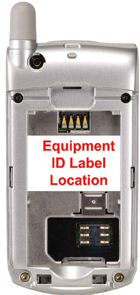
Rear View with Battery Removed to Show Equipment ID Label
