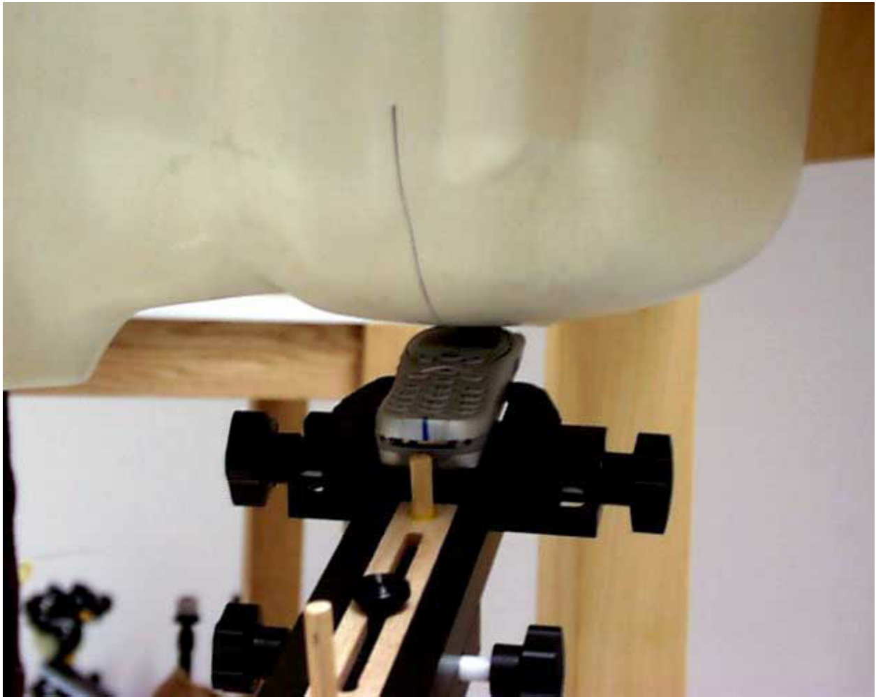
Figure 13. Bottom of Phone Seen in 15 Degree Tilt Testing Configuration
