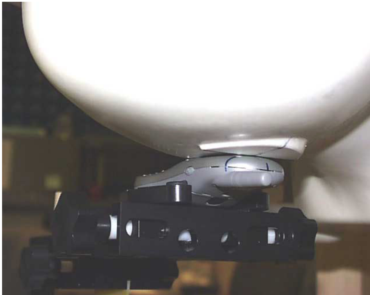
Figure 11. Top of Phone Seen in Cheek Touch Testing Configuration
