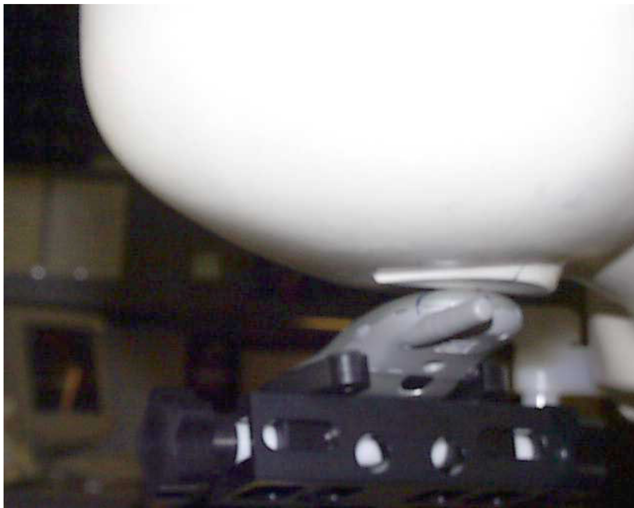
Figure 14. Top of Phone Seen in 15 Degree Tilt Testing Configuration
