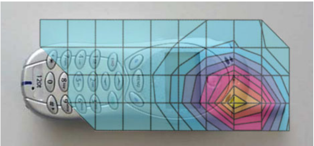
Figure 4. Typical 1900MHz 15 Degree Tilt SAR Contour Overlaid on Front of Phone
