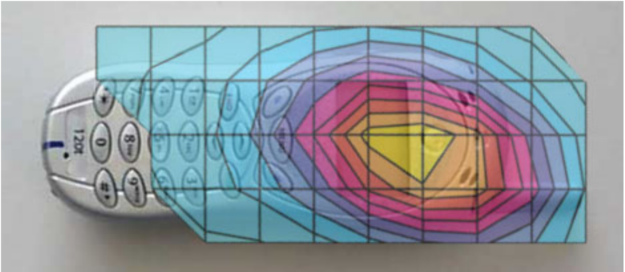
Figure 1. Typical 800MHz Cheek Touch SAR Contour Overlaid on Front of Phone
