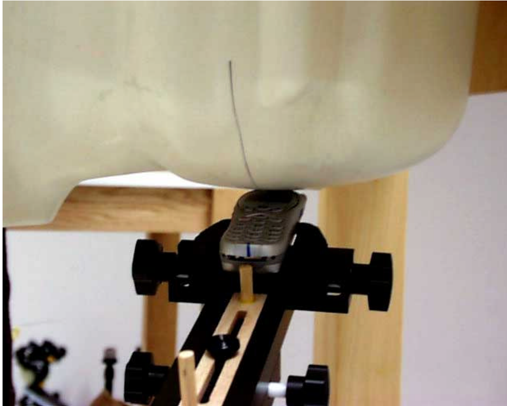
Figure 14. Front View of Phone Placed Against the Head (15° Tilt Position) with Antenna Fixed
