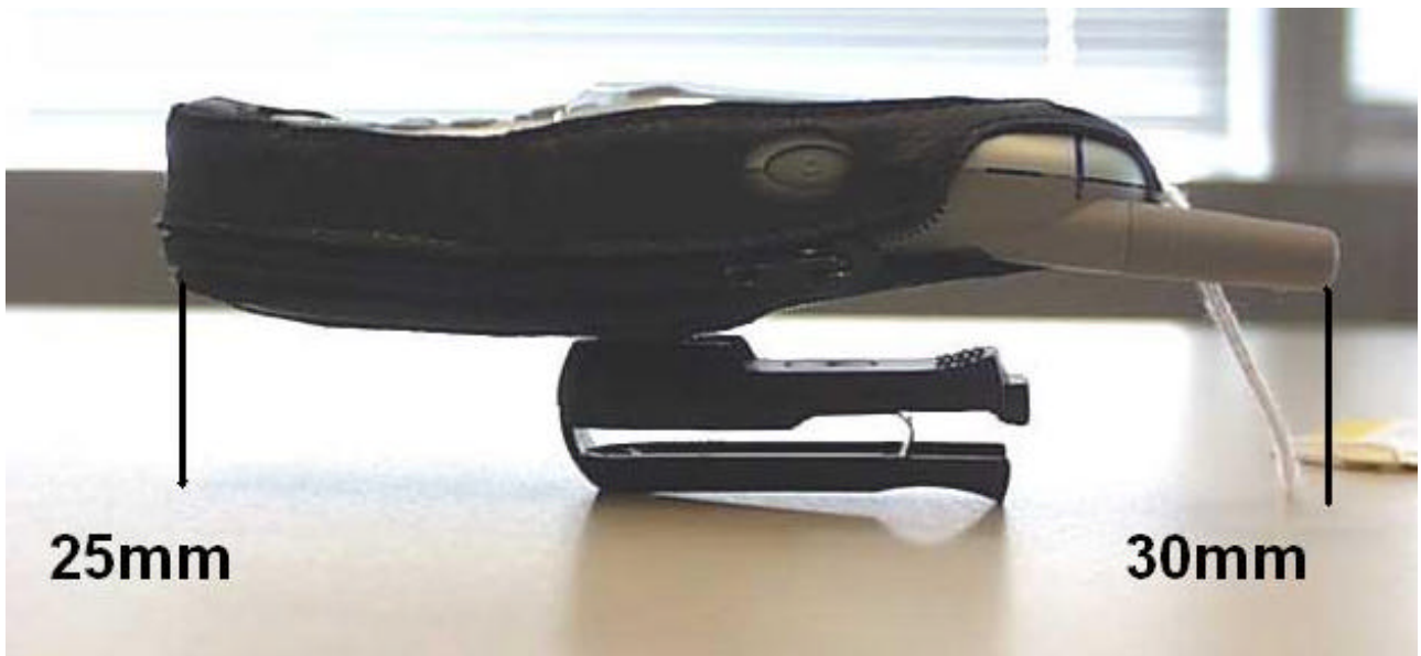
Figure 11. Distance of the Antenna (Fixed) to the Base of the Flat Phantom
