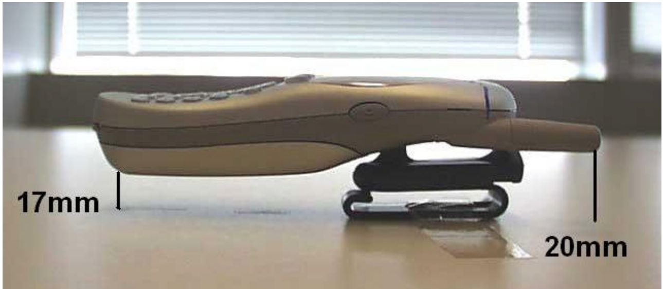
Figure 10. Distance of the Antenna (Fixed) to the Base of the Flat Phantom
