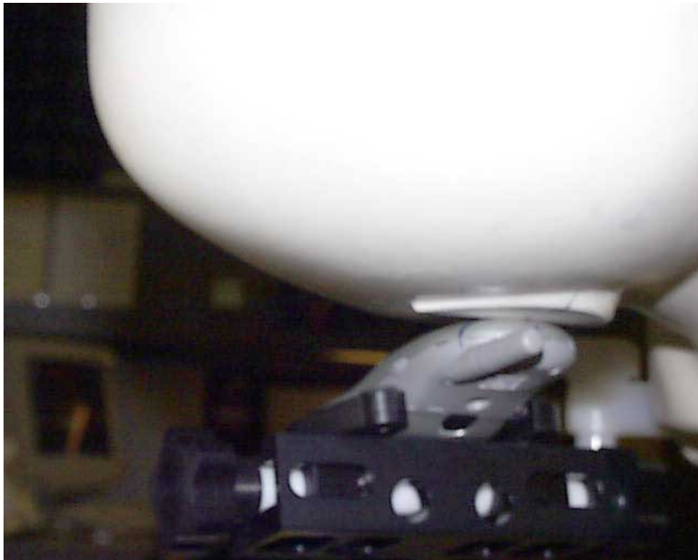
Figure 15. Back View of Phone Placed Against the Head (15° Tilt Position) with Antenna Fixed
