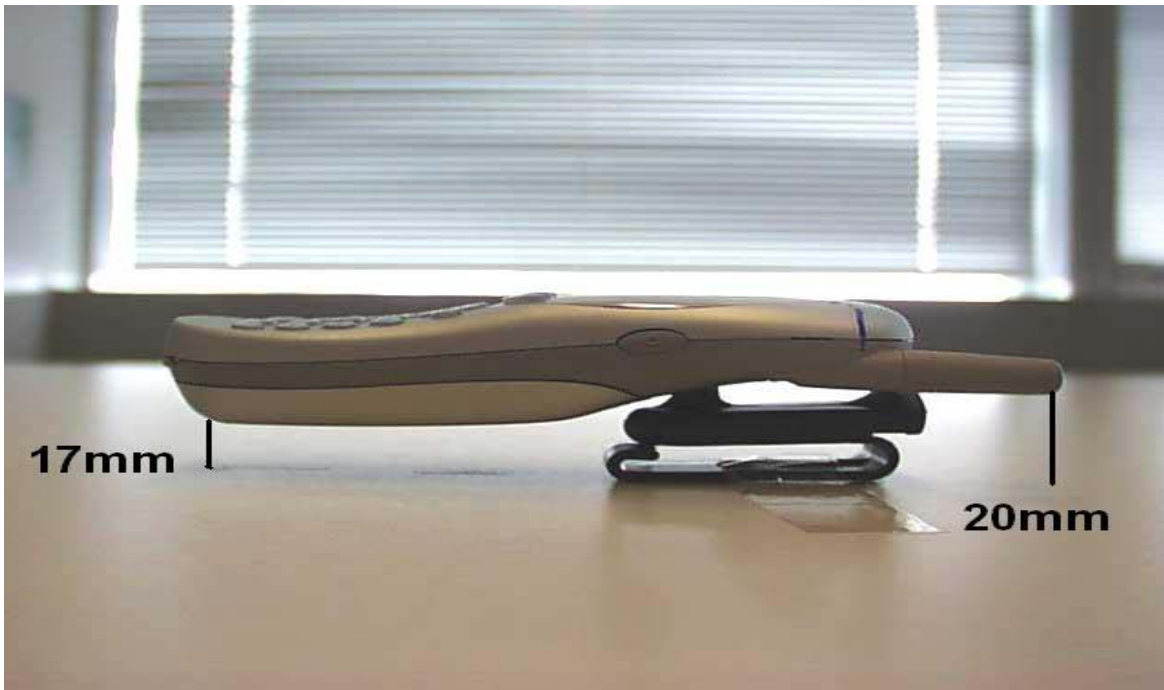
Figure 10. Separation Distance Provided from Plastic Belt Clip
