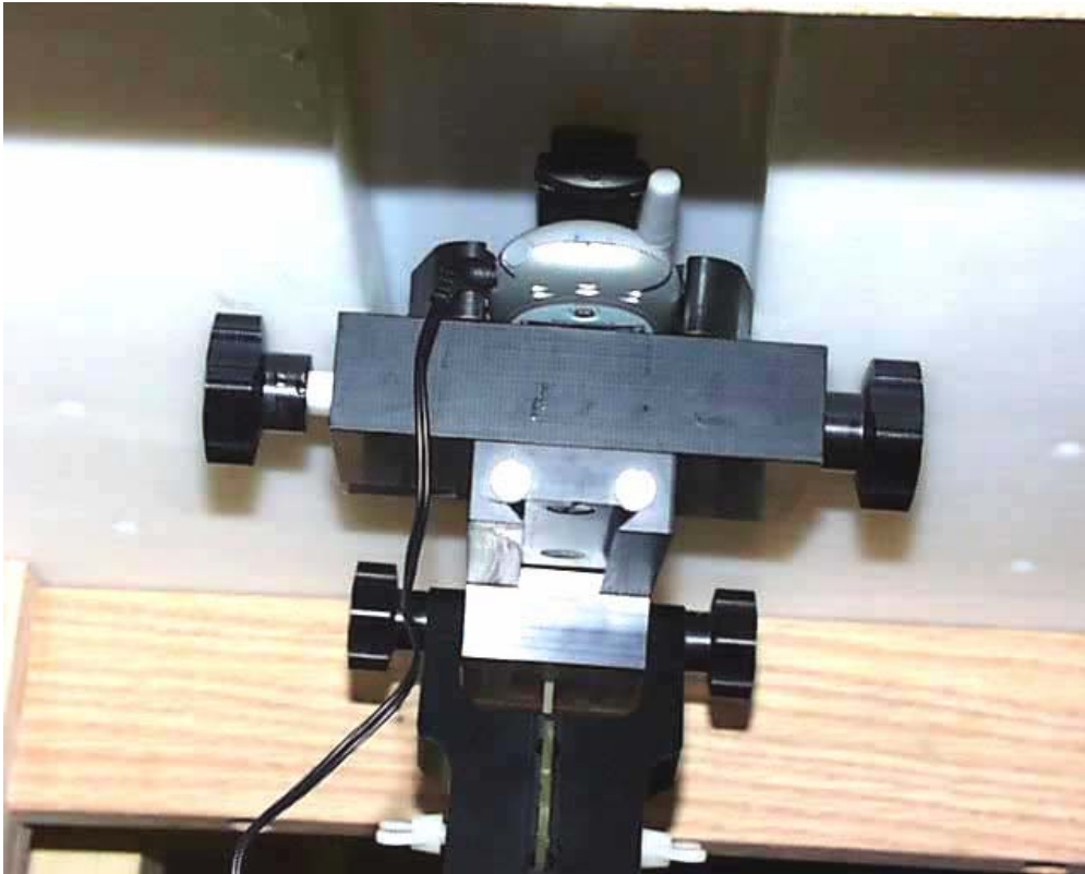
Figure 11. Phone with Belt Clip Placed under a Flat Phantom with Headset (Antenna Fixed)
