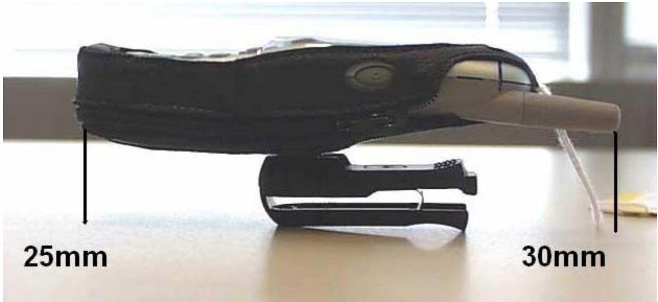
Figure 9. Distance of the Antenna (Fixed) to the Base of the Flat Phantom
