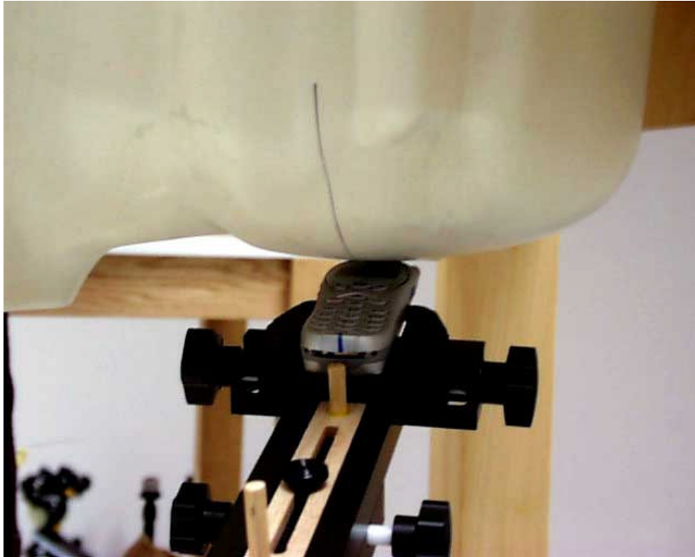
Figure 12. Front View of Phone Placed Against the Head (15° Tilt Position) with Antenna Fixed
