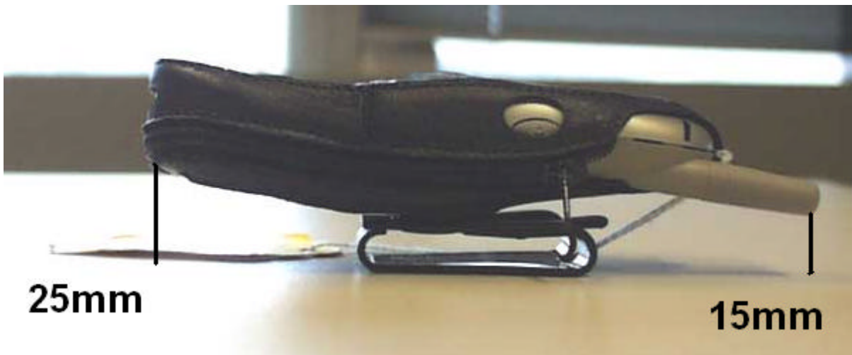
Figure 9. Distance of the Antenna (Fixed) to the Base of the Flat Phantom
