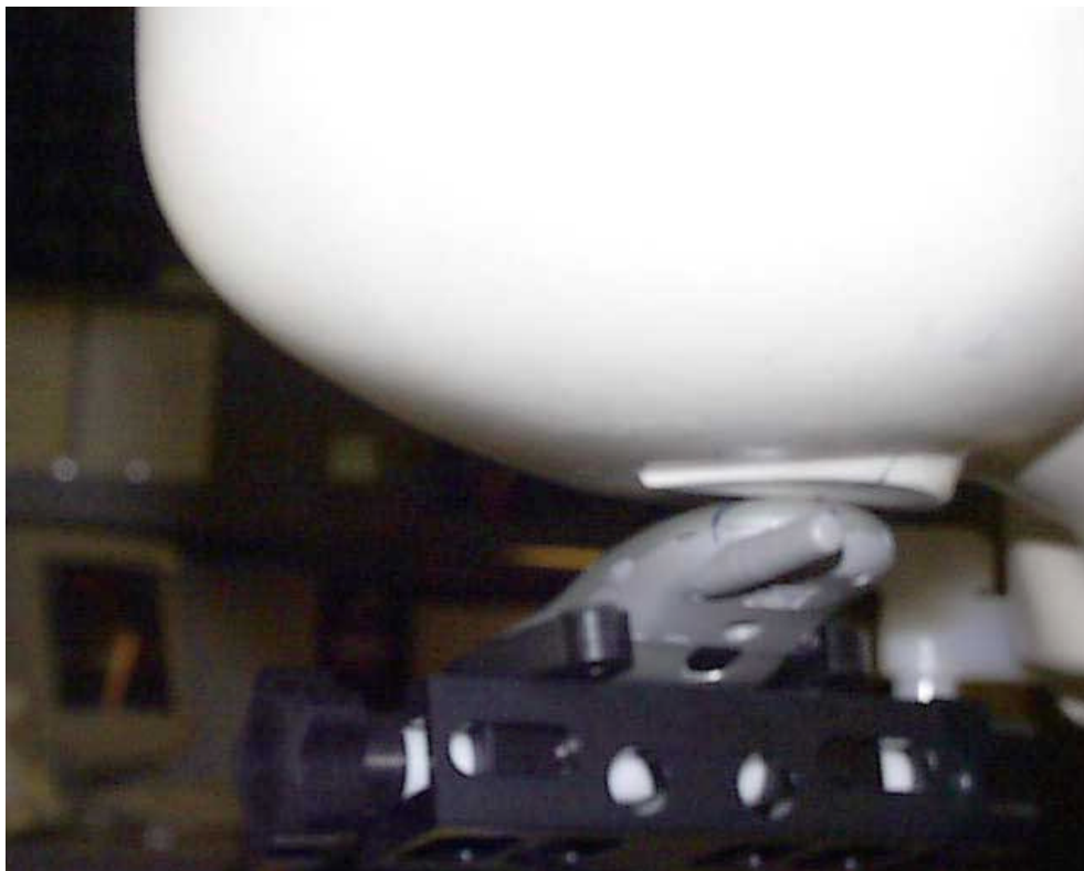
Figure 13. Back View of Phone Placed Against the Head (15° Tilt Position) with Antenna Fixed
