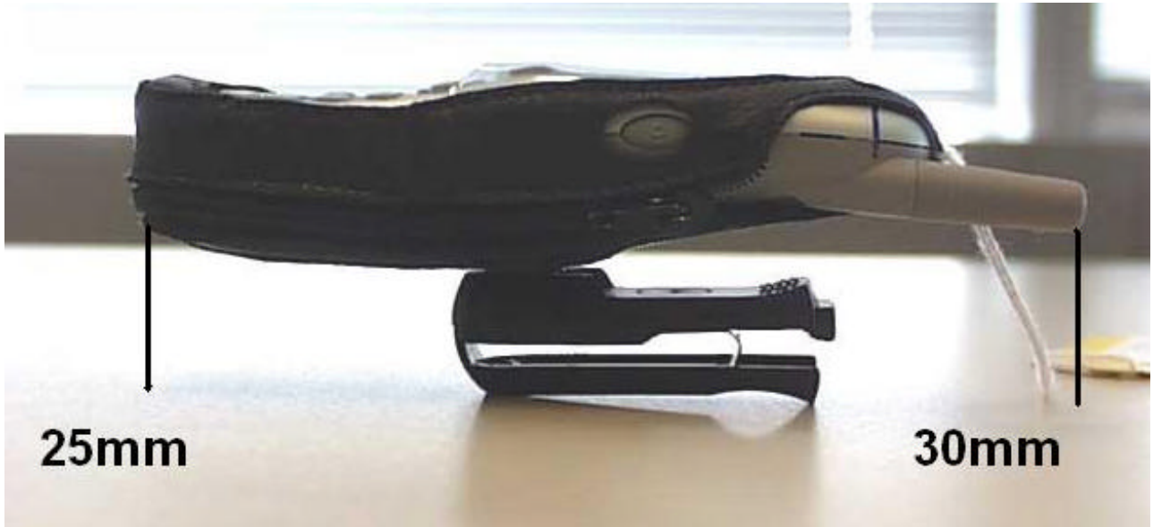
Figure 8. Distance of the Antenna (Fixed) to the Base of the Flat Phantom
