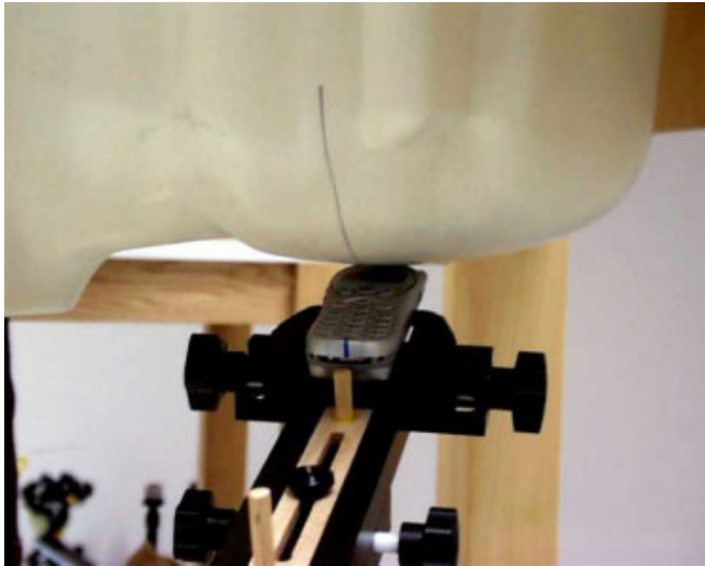
Figure 13. Front View of Phone Placed Against the Head (15° Tilt Position) with Antenna Fixed
