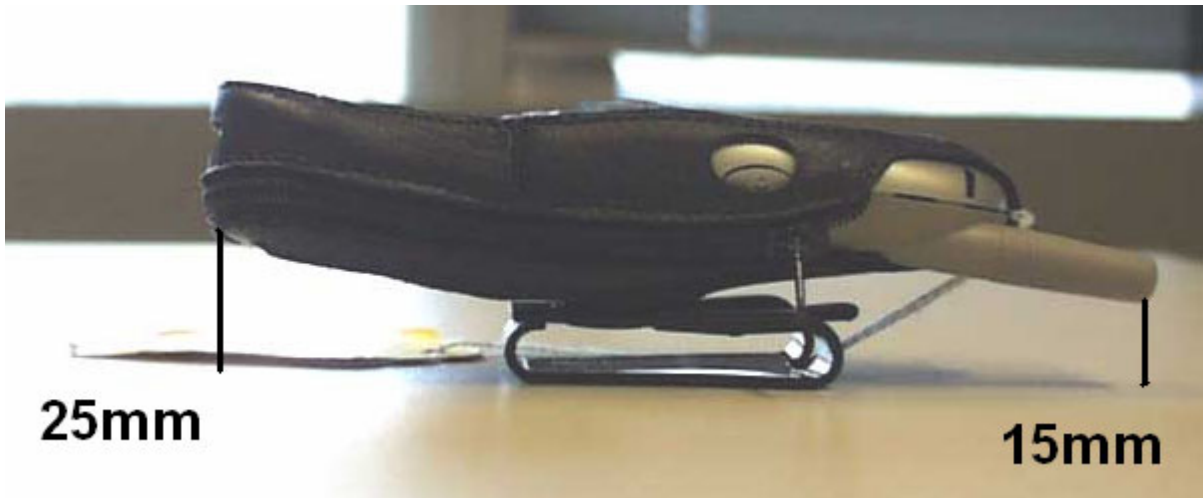
Figure 10. Distance of the Antenna (Fixed) to the Base of the Flat Phantom
