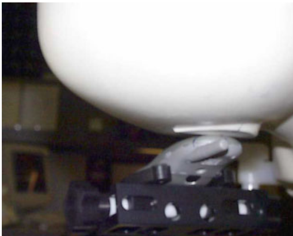
Figure 14. Back View of Phone Placed Against the Head (15° Tilt Position) with Antenna Fixed
