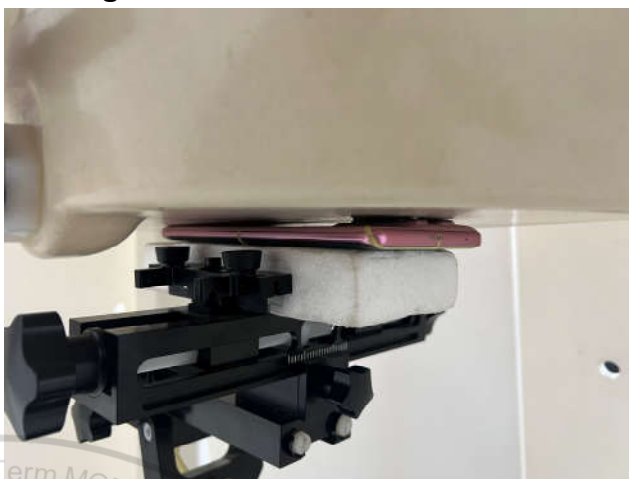
Back, Test Separation 0 mm
