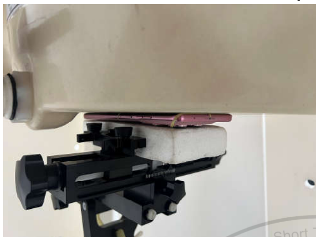
Front, Test Separation 0 mm
