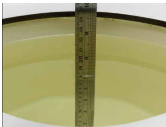
Fig 11.2 Photo of Liquid Height for Body SAR
