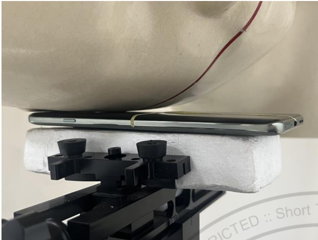
Right Cheek, Test Separation 0 mm
