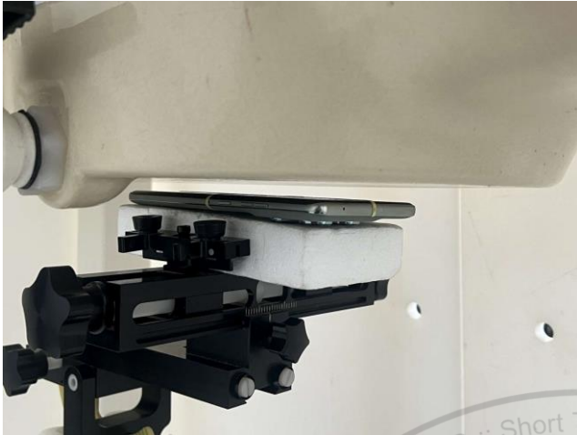
Front, Test Separation 10 mm
