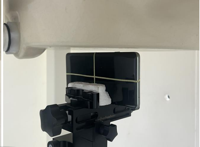
Left Side, Test Separation 5 mm
