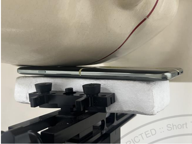
Right Cheek, Test Separation 0 mm
