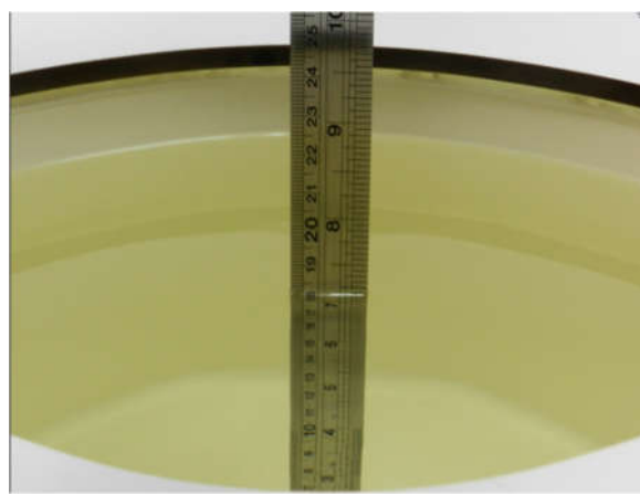
Fig 11.2 Photo of Liquid Height for Body SAR
