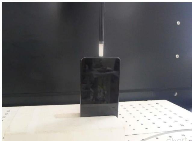
Top Side, Test Separation 2 mm
