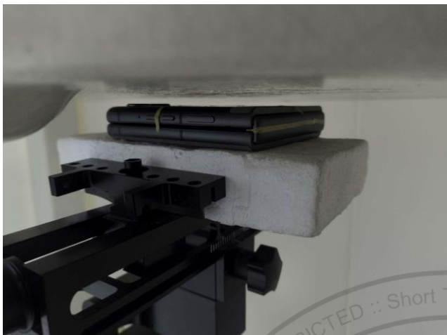
Front, Test Separation 5 mm
