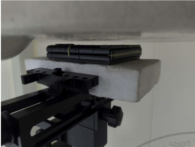
Front, Test Separation 5 mm
