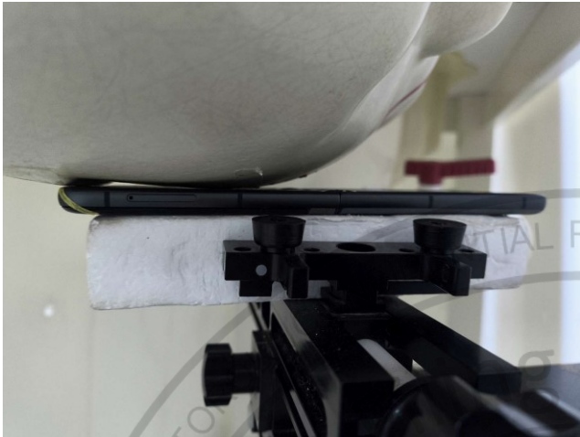
Right Cheek, Test Separation 0 mm
