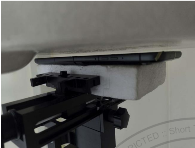
Front, Test Separation 5 mm
