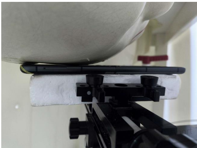
Right Cheek, Test Separation 0 mm
