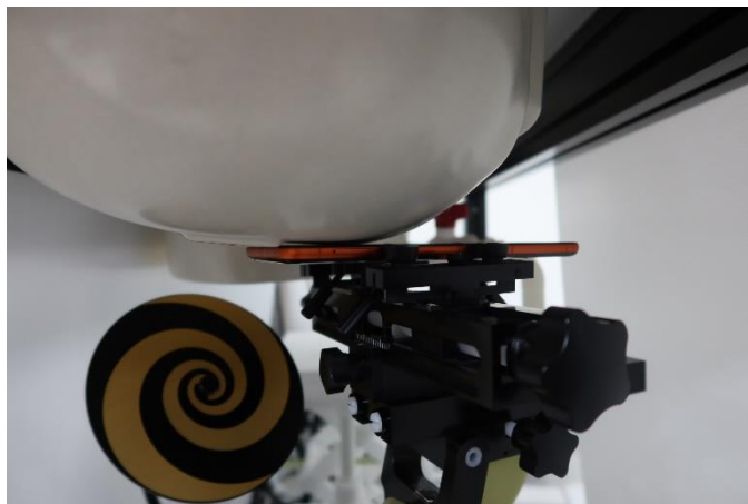
Right Cheek, Test separation 0mm
