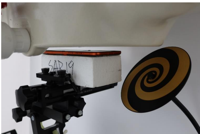
Front, Test separation 5mm
