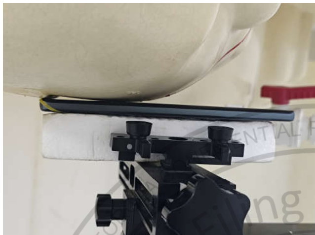
Right Cheek, Test Separation 0 mm
