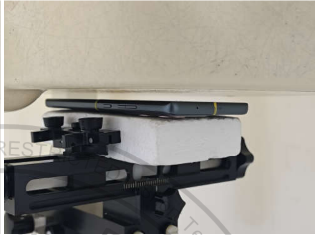
Front, Test Separation 7 mm
