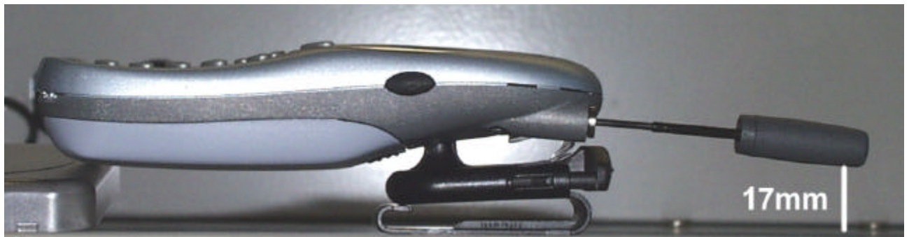
Figure 10. Distance Provided by Belt-Clip with Antenna Extended
