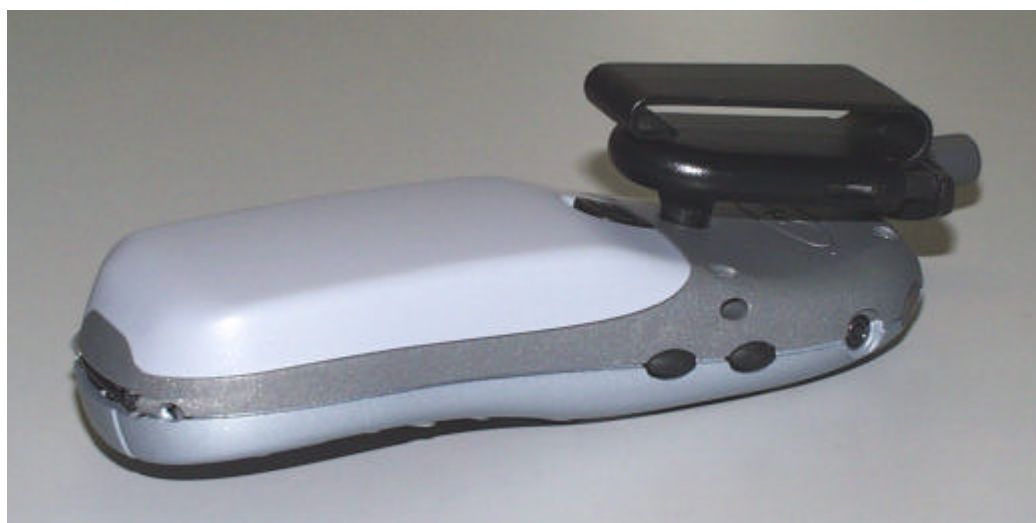
Figure 8. Back of Phone with Belt-Clip Attached.
