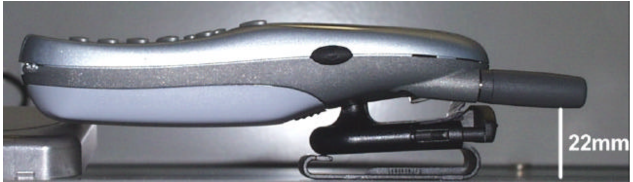
Figure 9. Distance Provided by Belt-Clip with Antenna Retracted
