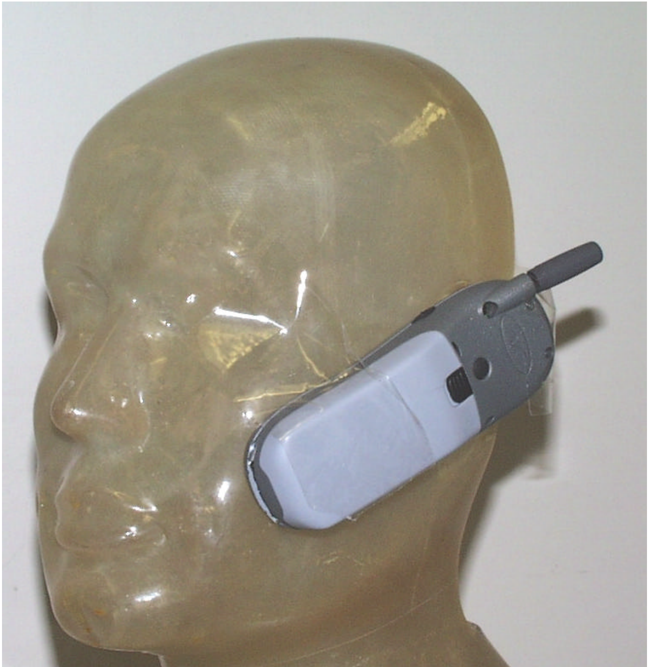
Figure 6. Phone Against Phantom Head with Antenna Retracted.
