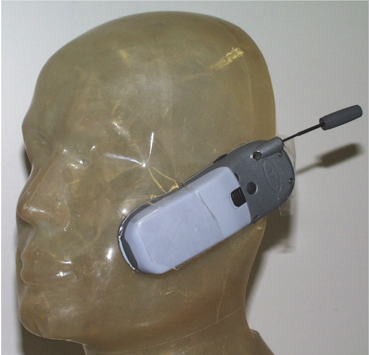
Figure 5. Phone Against Phantom Head with Antenna Extended
