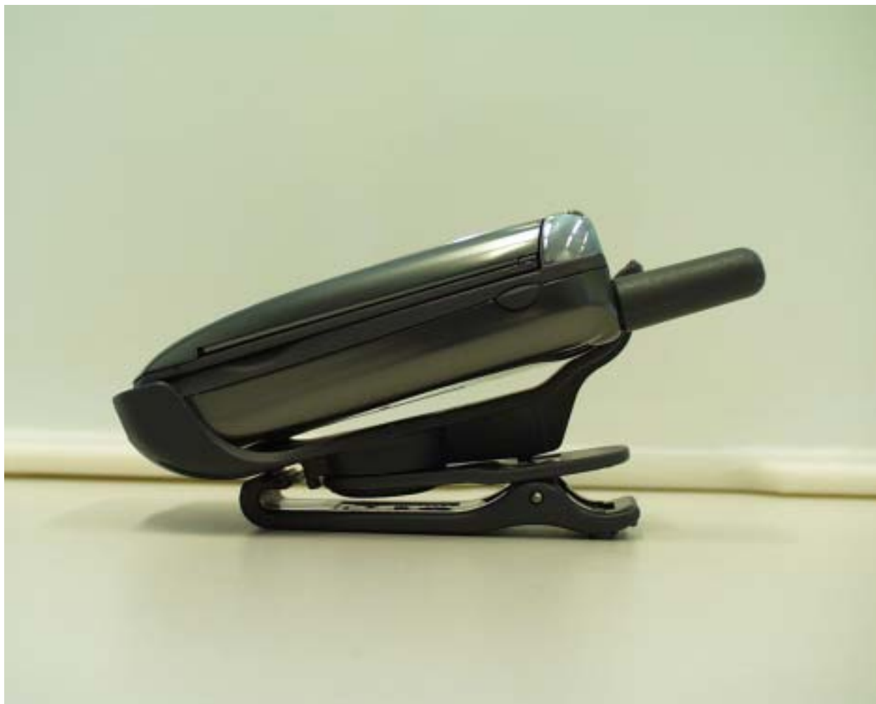
Figure 9. Separation Distance of 33 mm from Tip of Antenna to Flat Phantom and 10 mm from the bottom of the clip when rotated 0°.
