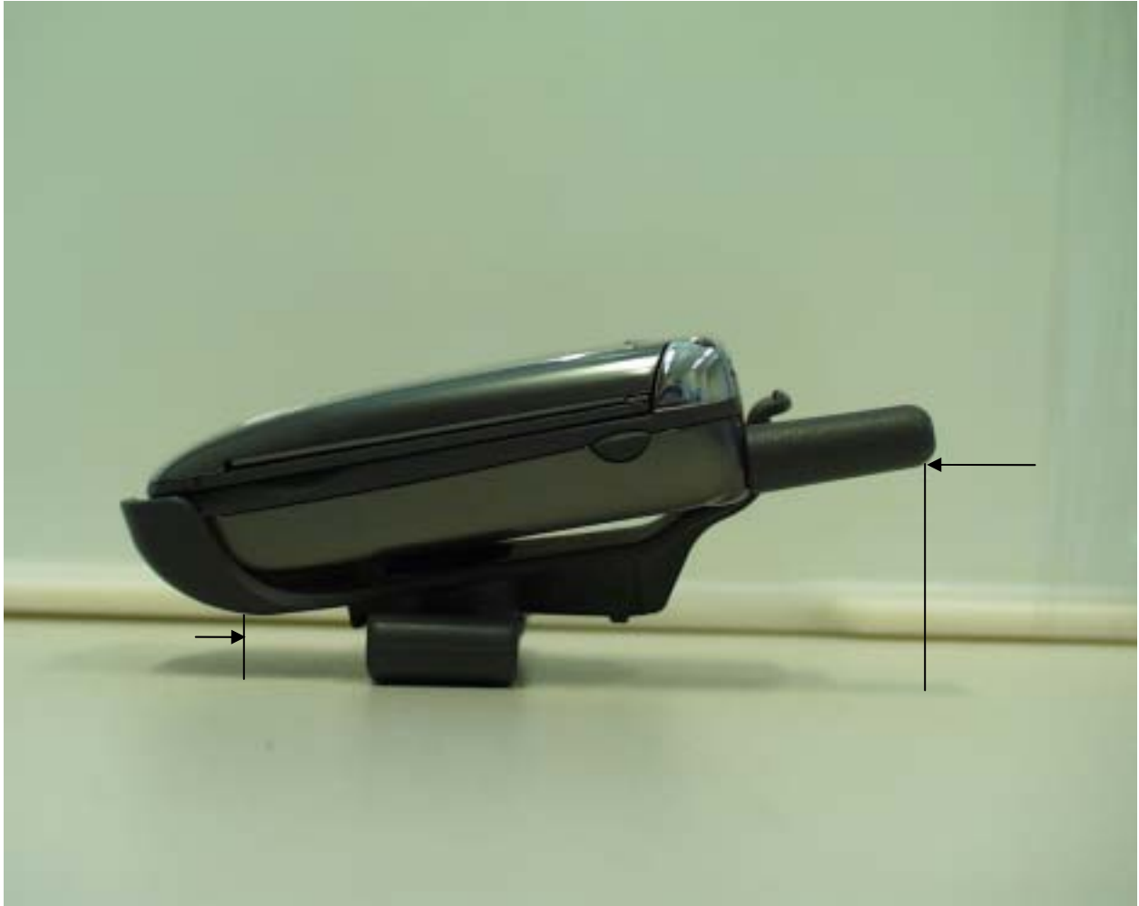
Figure 8. Separation Distance of 25 mm from Tip of Antenna to Flat Phantom and 8 mm from the bottom of the clip when rotated +90° (Clockwise Direction)
