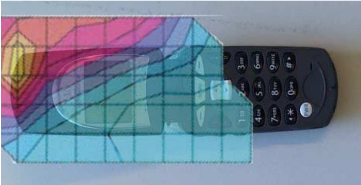
Figure 3. Typical 800MHz Head Adjacent Contour Overlaid on Phone (15 ° Tilt)
