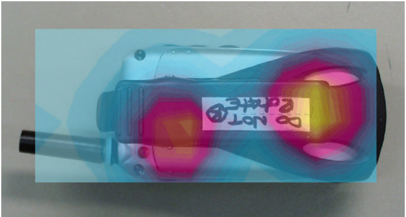
Figure 10. Showing Typical 1900MHz contour plot overlaid on Belt Clip
