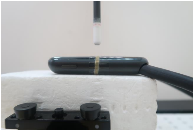
Front Surface, Test Separation 14 mm
