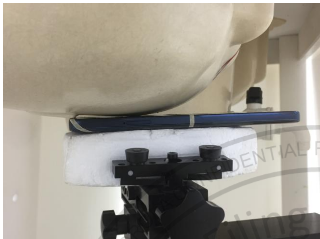
Right Cheek, Test Separation 0 mm
