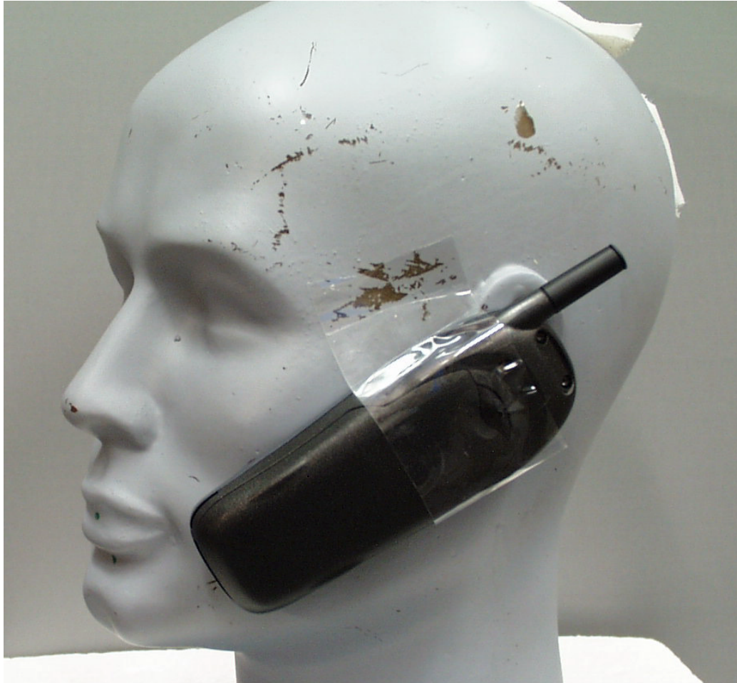
Figure 3. Phone against side of Phantom Head with Antenna Retracted
