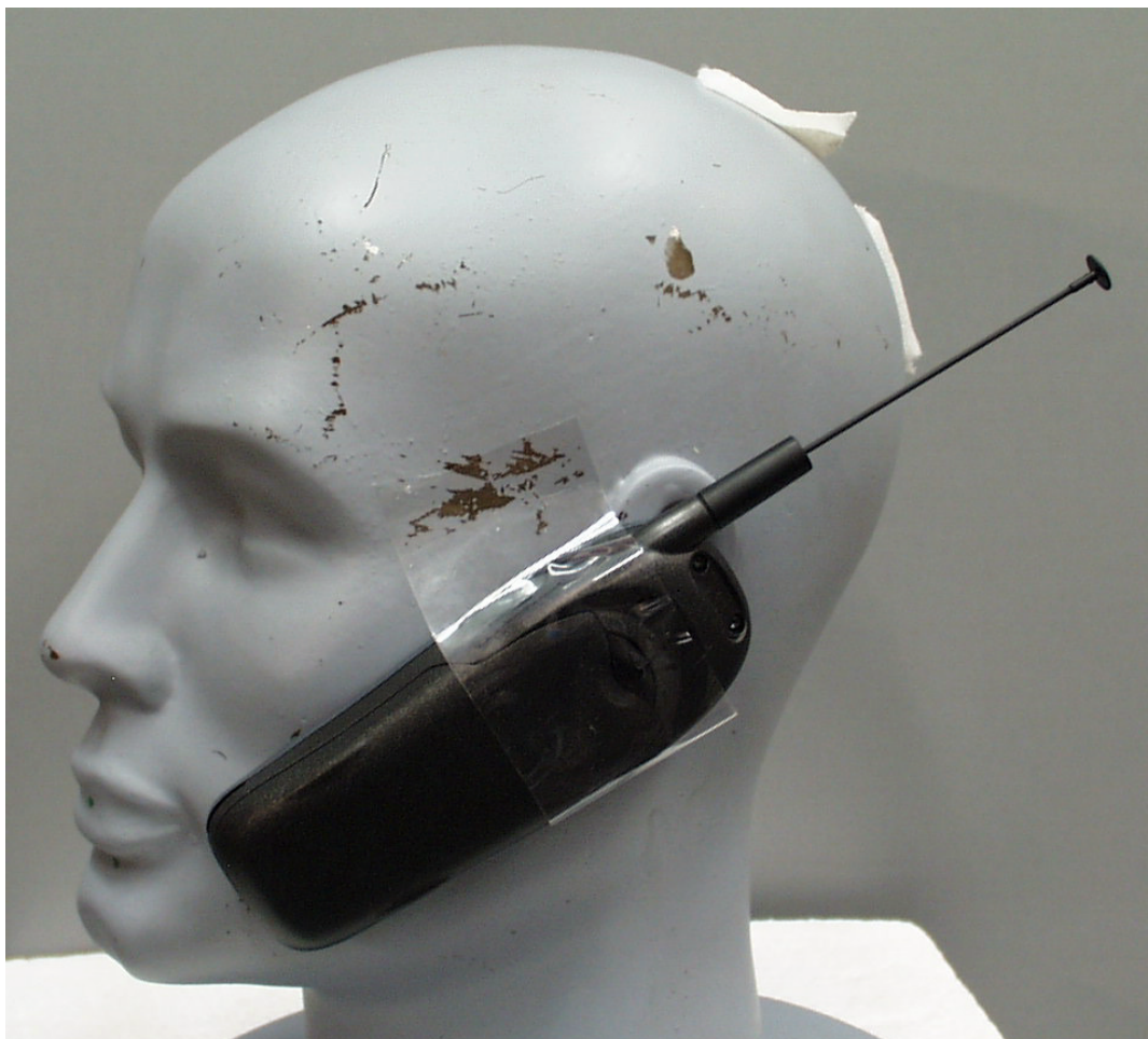
Figure 4. Phone against side of Phantom Head with Antenna Extended
