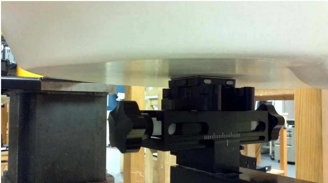
Figure 2: Back Surface of DUT toward Phantom, 0 mm Separation
