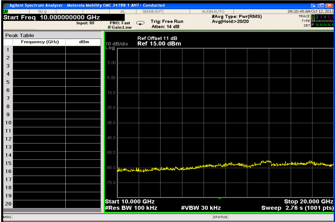
Conducted Spurious Emissions 10-20 GHz (Low Channel)
