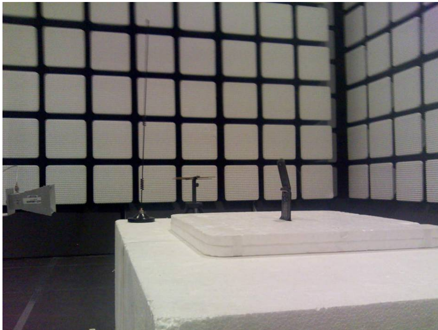
23059-1, IHDP6KL1 setup in semi-anechoic chamber – right view (18 GHz – 26.5 GHz)
