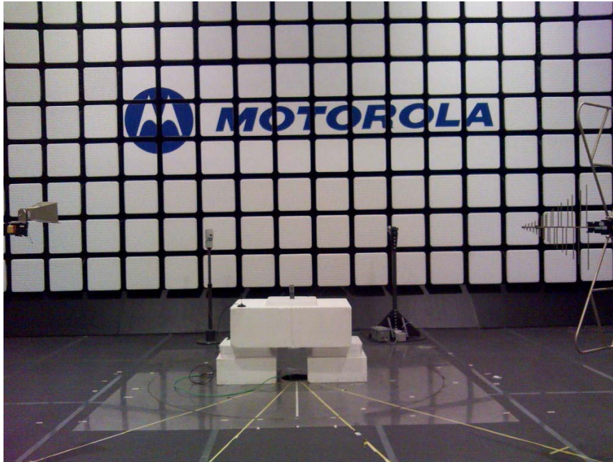
23059-1, IHDP6KL1 setup in semi-anechoic chamber – front view (30 MHz – 18 GHz)
