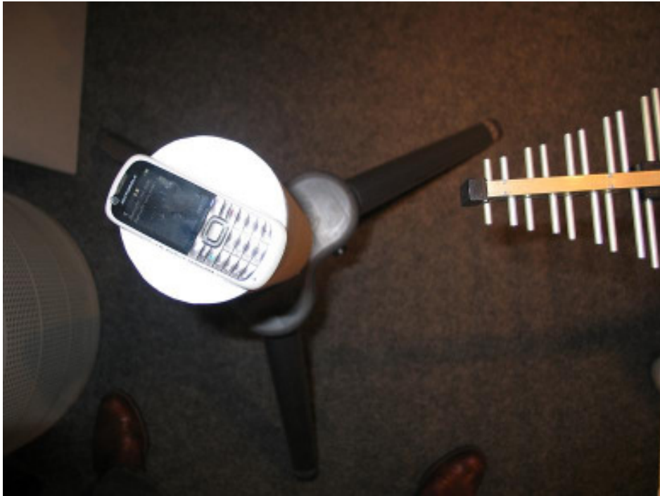
21943-1, IHDP6JL1 Check for maximum radiation at position X
