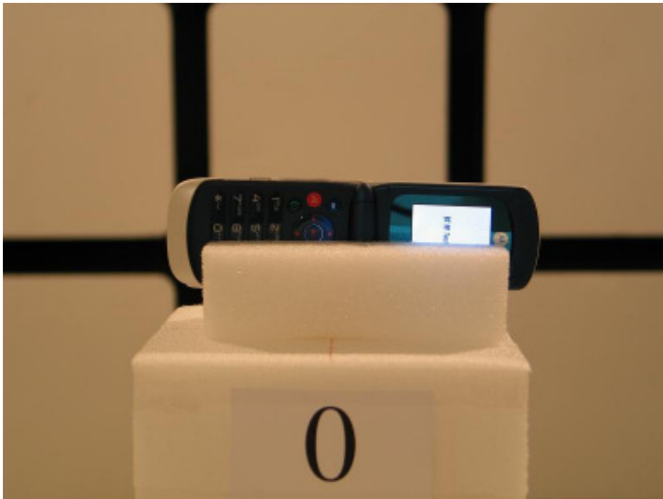
21844-1, IHDP6JJ1 placed in test position Y - Open
