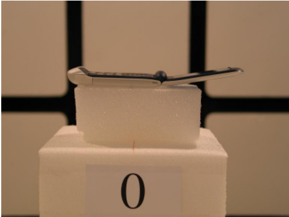
21844-1, IHDP6JJ1 placed in test position X - Open
