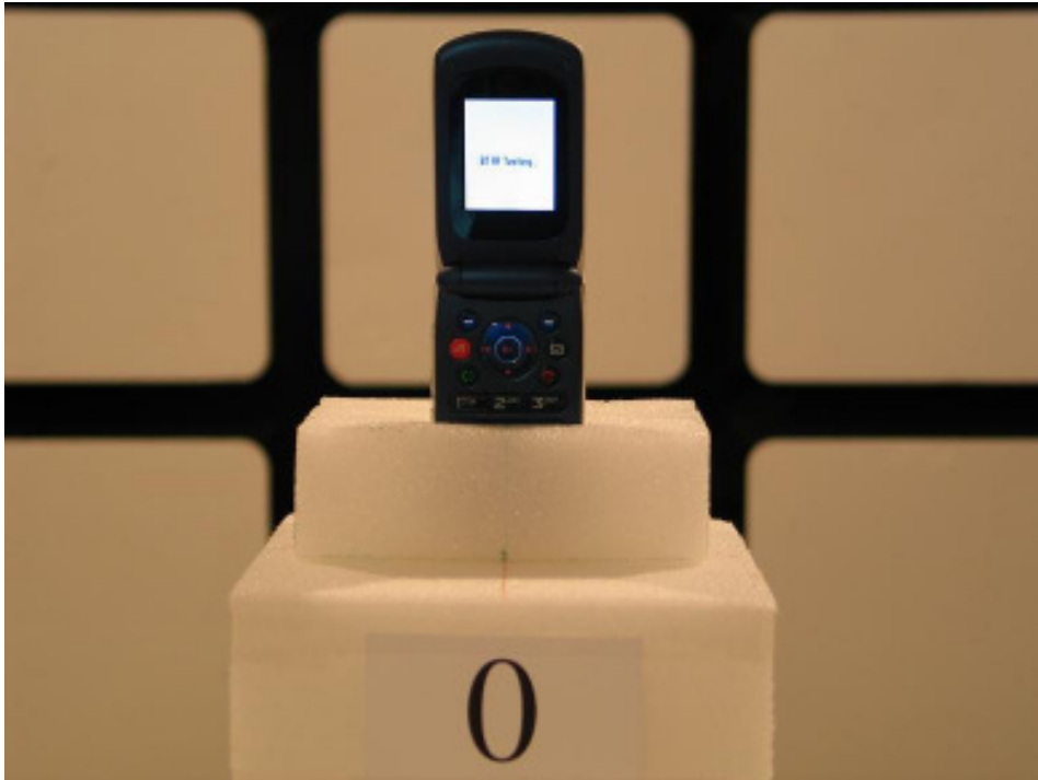
21844-1, IHDP6JJ1 placed in test position Z - Open
