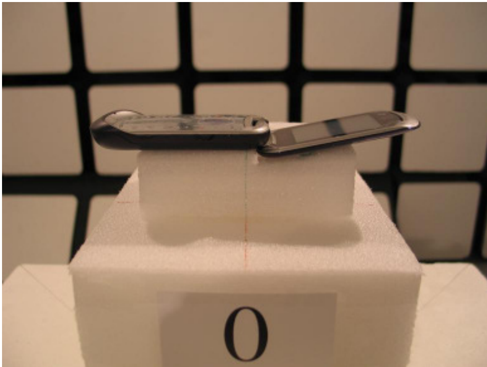
21835-1, IHDP6JH1 placed in test position X - Open
