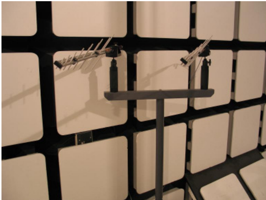
21835-1, IHDP6JH1 setup in semi-anechoic chamber – link antennas
