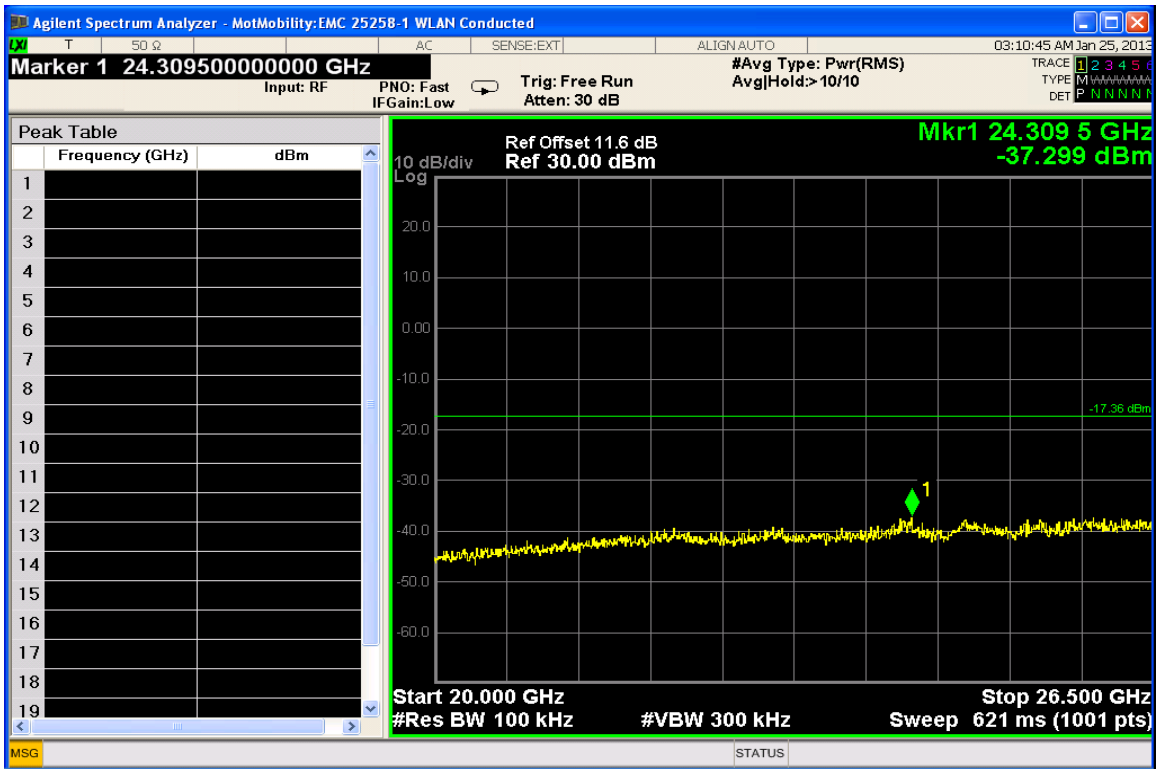
Conducted Spurious Emissions 20GHz-26.5GHz (Mid Channel)
