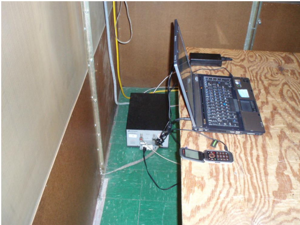
POWERLINE CONDUCTED EMISSIONS TEST SET UP PHOTO
