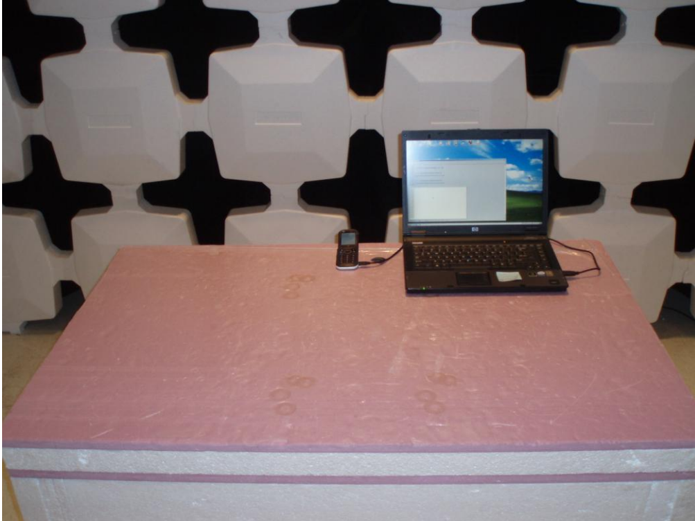
RADIATED EMISSIONS TEST SETUP PHOTO
