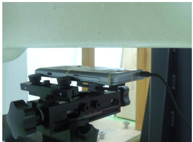
Rear Face of EUT with 2.5 cm Gap (Body-Worn Mode)
