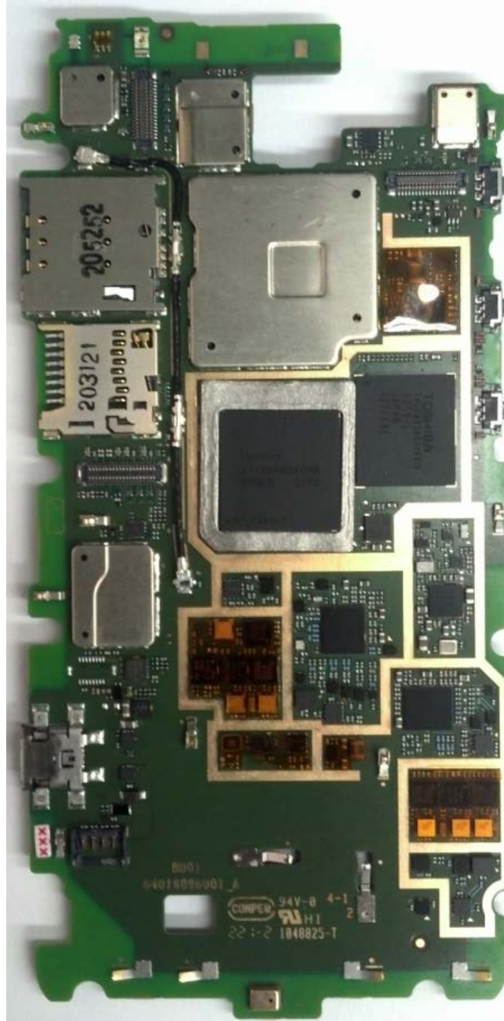
Photograph 9-1: Front side view of the device's PC Board, Shields in place.
