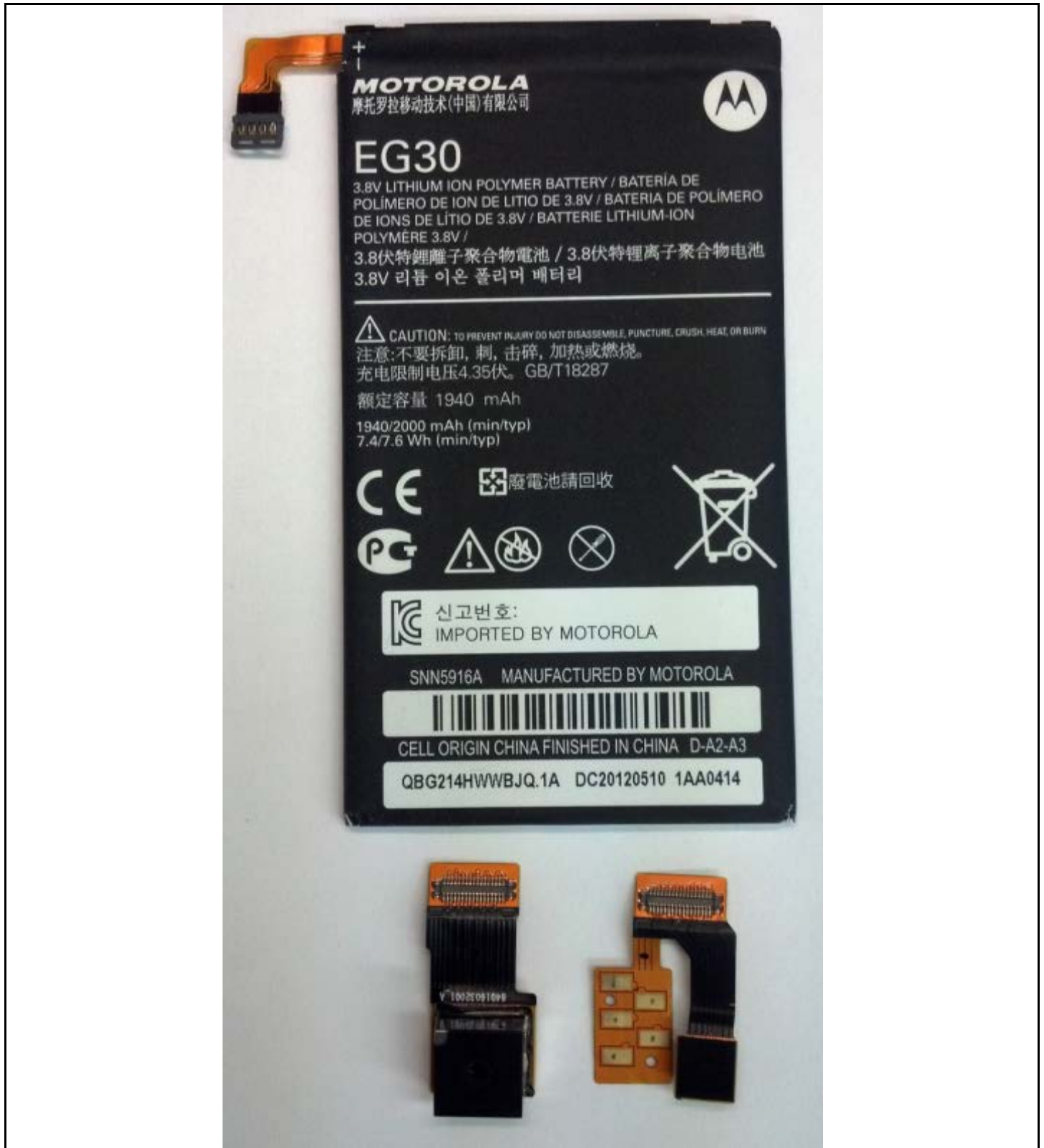
Photograph 9-5: Internal Battery and Flex Circuits.
