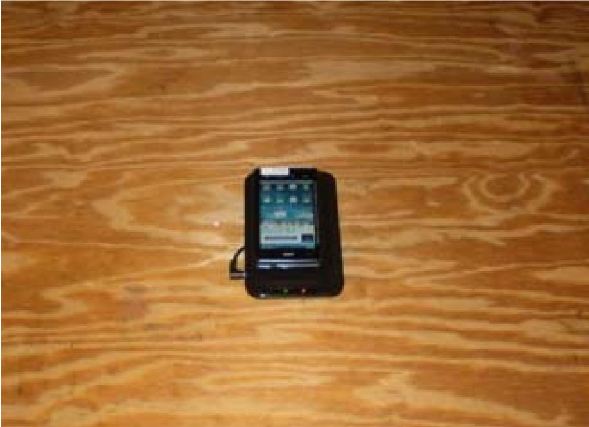
Tx Radiated – Part 15 Unintentional Radiator with Inductive Charging Door and Charging Pad
