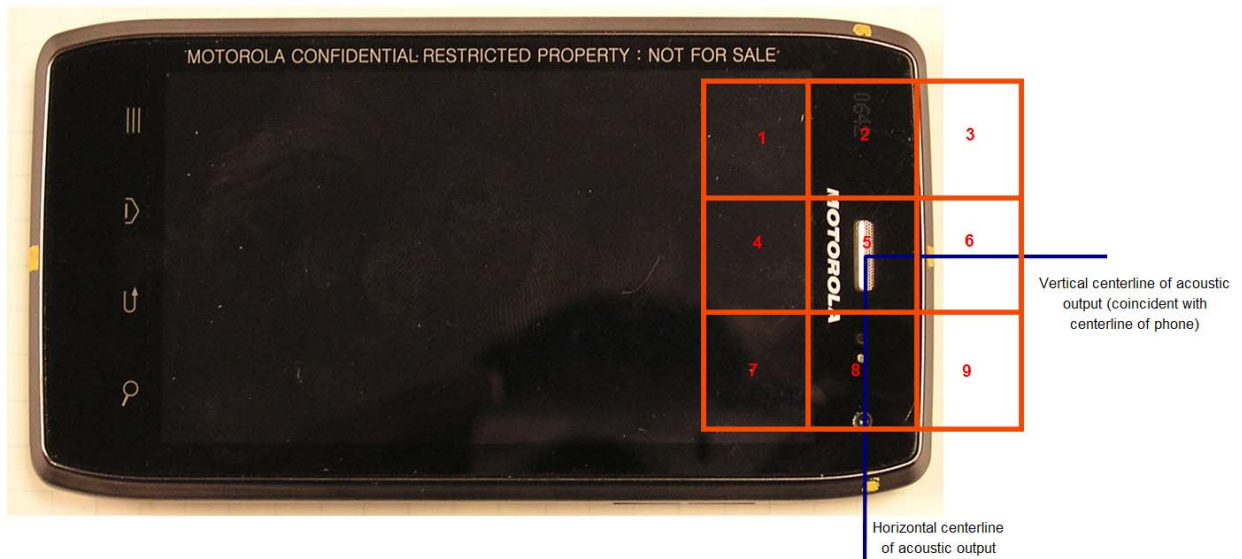
Figure 2. Phone Front - Orientation and Measurement Plane for RF Emissions Testing
