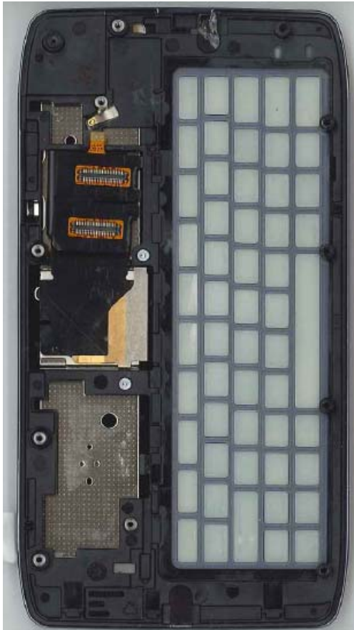
Rear Housing and Main Board Removed
