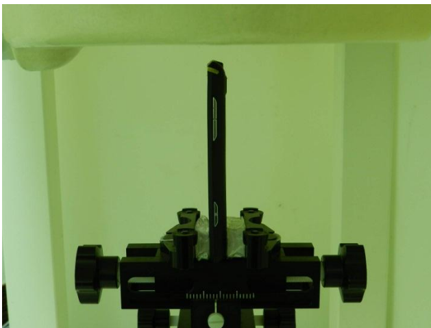
Top Side of the DUT with Phantom 1 cm Gap
