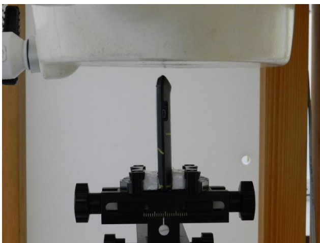
Bottom side of the DUT with Phantom 1 cm Gap (DUT without Earphone)
