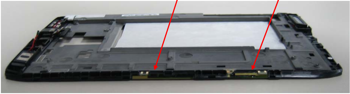
GPS and BT/WiFi Antenna Location
