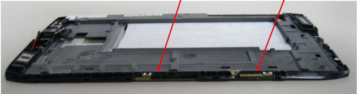
GPS and BT/WiFi Antenna Location
