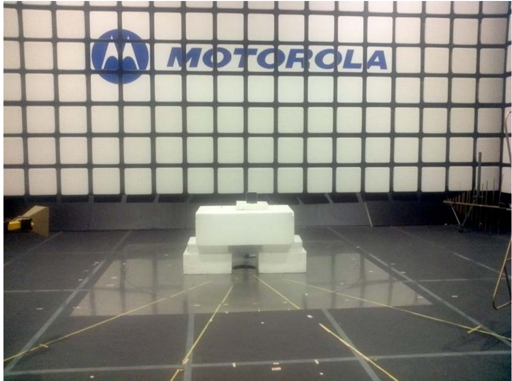
BJ EMC lab Radiated Emissions
