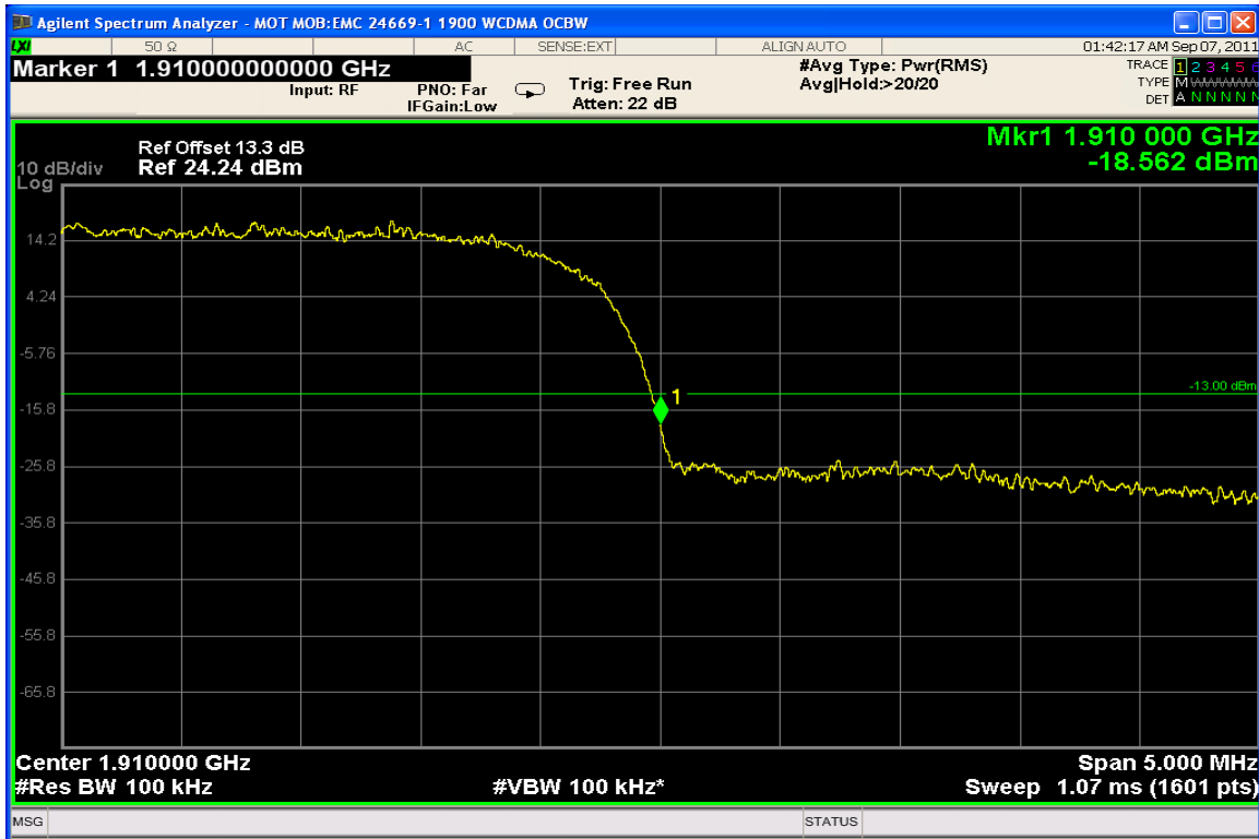
WCDMA 1900 – Upper Band Edge – Channel 9538 (1907.60 MHz)
