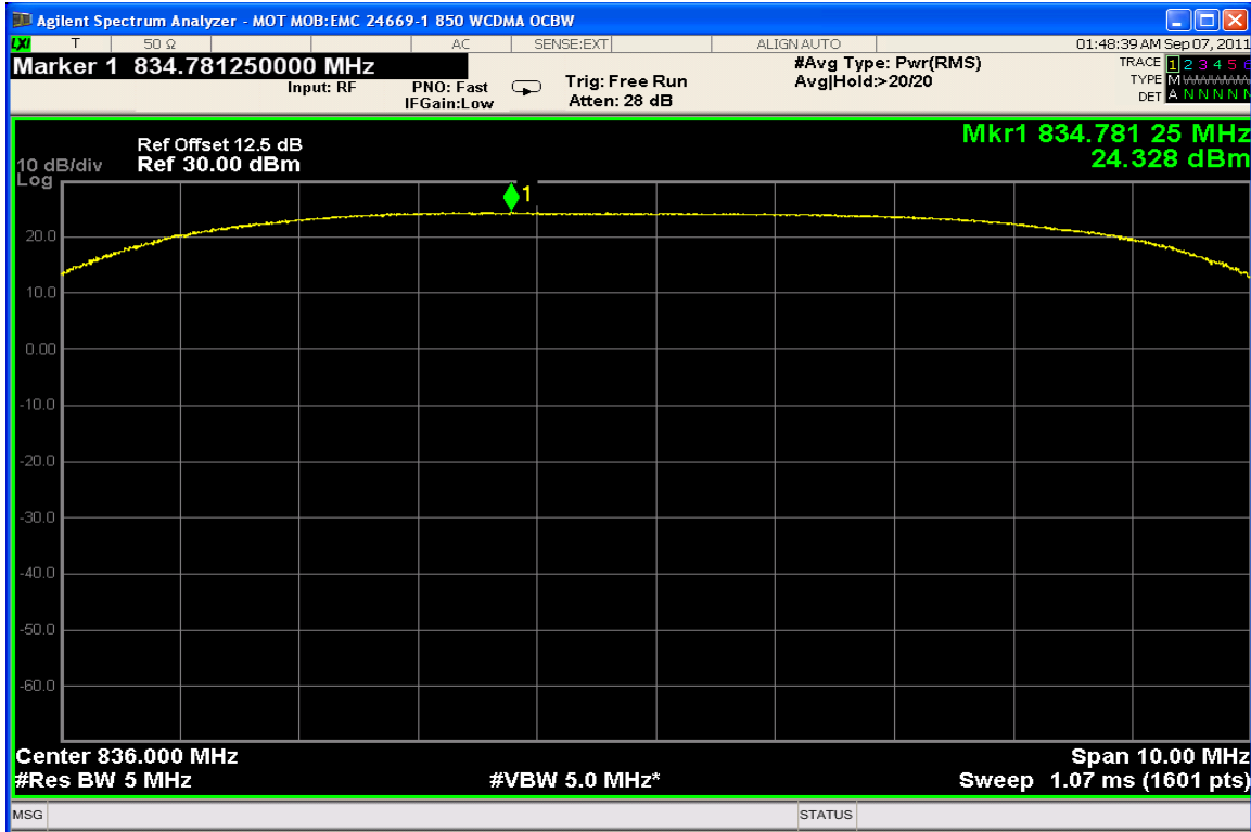
WCDMA 850 – Reference Level Plot – Channel 4180 (836.00 MHz)
