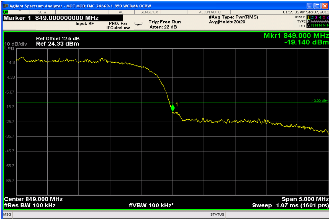
WCDMA 850 – Upper Band Edge – Channel 4233 (846.60 MHz)
