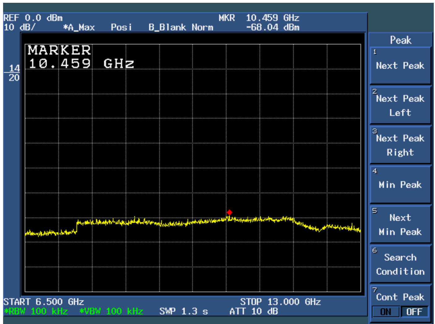
Figure 6d.7-12: Plot of spurious conducted emissions 6.5 GHz – 13.0 GHz (Hopping Function Channel Enabled).
