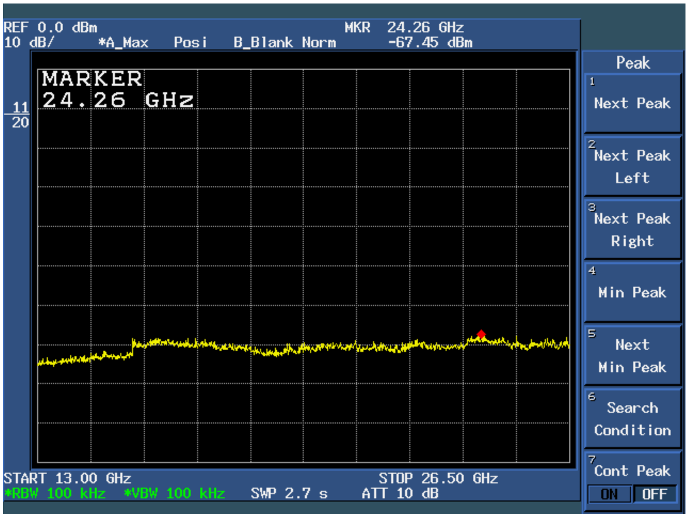
Figure 6d.7-13: Plot of spurious conducted emissions 13 GHz – 26.5 GHz (Hopping Function Channel Enabled).
