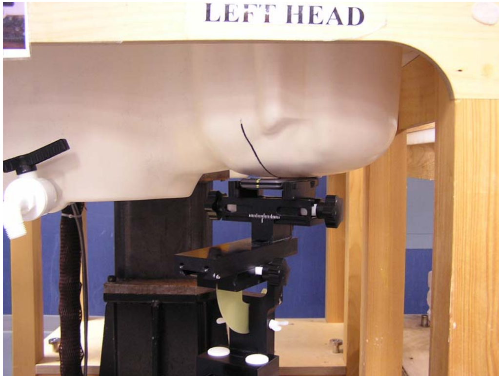
Figure 3: Cheek Position, Front of Head of Phantom
