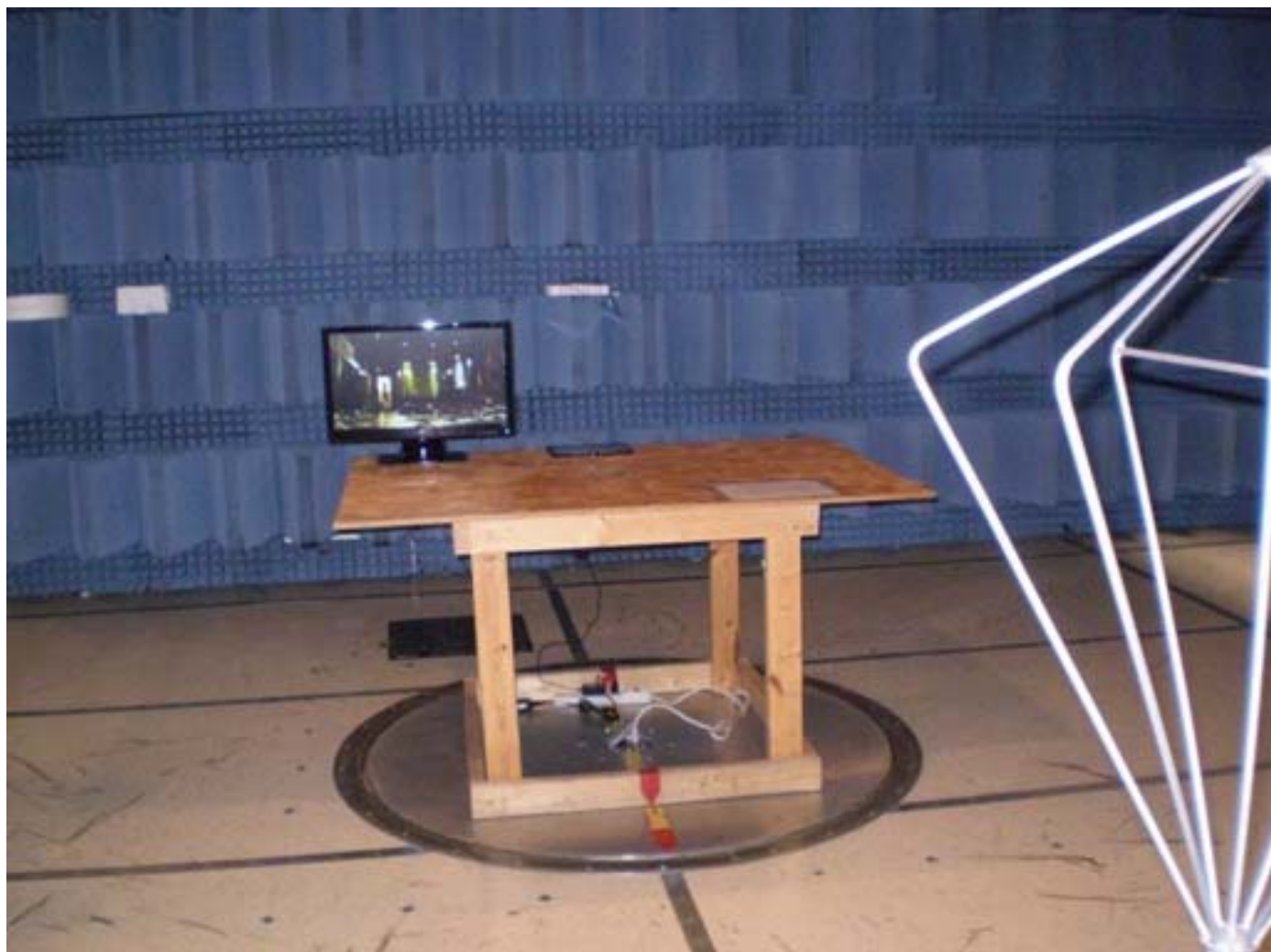
Figure 7c2-1: Spurious Radiations (Part 15 Computing Device).
