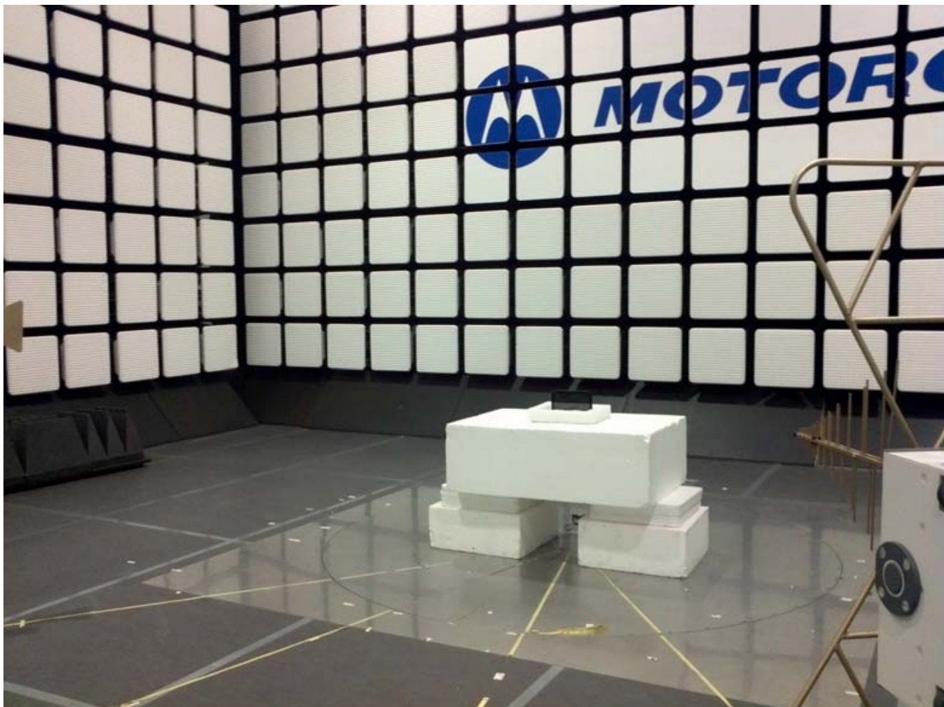
Figure 7c1-1: TX Radiated Emissions Configuration.
