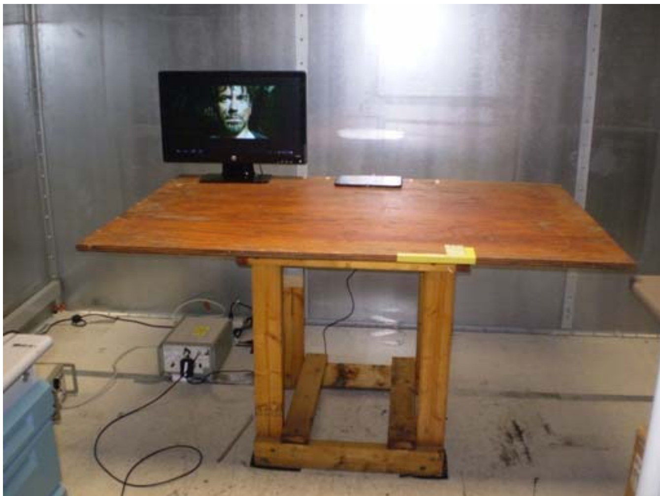
Figure 7c3-1: Test Configuration – AC Line (Part 15 Computing Device).
