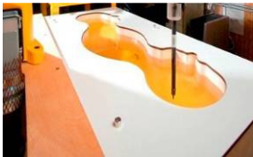
Figure 6-2 SAM Phantom with Simulating Tissue
